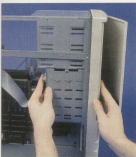
Any computer is pretty useless without a floppy drive. So, it's time to put the floppy disk into the tower case's drive cage and slot it into position
